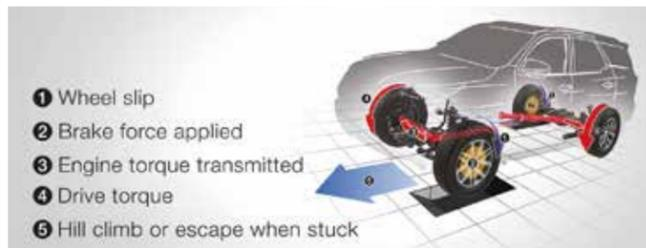
ACTIVE TRACTION CONTROL (A-TRC)\*\*: WHEN DRIVING OFF-ROAD OR IN SLIPPERY CONDITIONS, A-TRC APPLIES BRAKE PRESSURE TO PREVENT WHEELS FROM SPINNING DURING ACCELERATION.
