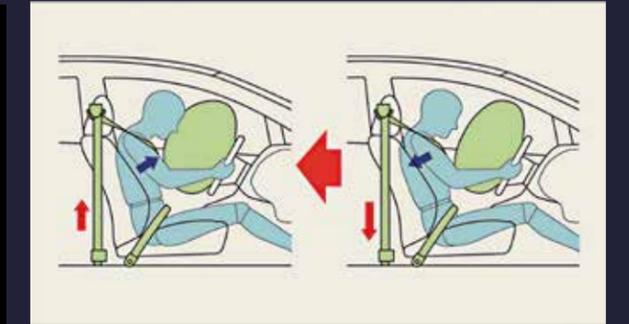
3-POINT ELR FRONT SEATBELTS WITH PRETENSIONER AND FORCE LIMITER
