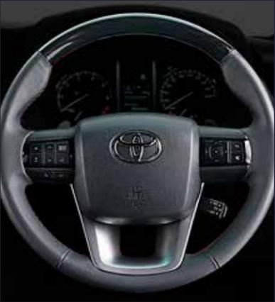
A SIX-SPEED SEQUENTIAL GEARBOX WITH PADDLE SHIFTERS IS STANDARD ON ALL FORTUNER VARIANTS. ADDITIONAL SMOOTHNESS HAS BEEN ACHIEVED THANKS TO THE ADDITION OF VARIABLE FLOW CONTROL POWER STEERING, WHICH IMPROVES STEERING FEEL BY PROVIDING MORE REALISTIC INPUT IN RELATION TO THE VEHICLE SPEED, WHILE ALSO BEING MORE FUEL EFFICIENT THAN THE STANDARD POWER STEERING SYSTEMS.
