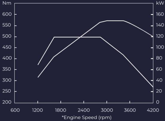
THE NEW GENERATION 2.8-LITRE DIESEL ENGINE (LGD-FTV) HAS BEEN FINE-TUNED FOR INCREASED POWER AND FUEL EFFICIENCY. THE VARIABLE NOZZLE TURBOCHARGER AND THE INTERCOOLER HAVE BEEN IMPROVED, RESULTING IN INCREASED POWER AND TORQUE PRODUCTION, AS WELL AS IMPROVED FUEL ECONOMY.
