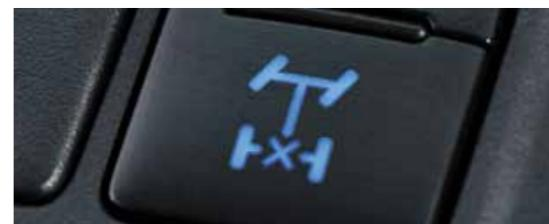
THE REAR DIFFERENTIAL LOCK SYSTEM HELPS SECURE TRACTION WHEN DRIVING IN MUDDY TERRAIN, OR IN THE UNLIKELY SITUATION WHEN THE VEHICLE IS STUCK. THE VEHICLE IS EQUIPPED WITH A SOLENOID SWITCH DIFFERENTIAL LOCK SYSTEM.
